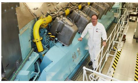
The dual-fuel engine on AIDAprima. LNG flows through the yellow pipes to the cylinders.
